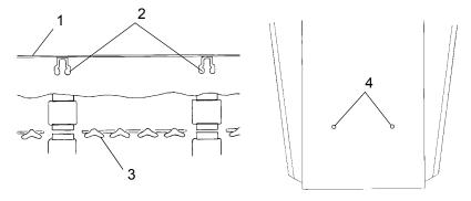
**NOTICE:** Whenever wear strips are relocated, be sure there's adequate stud clearance to the heat exchangers. Lack of clearance may result in damage to heat exchangers.
